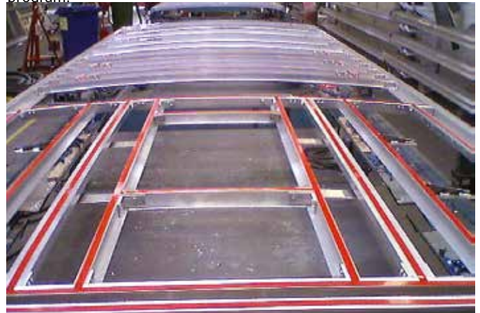
Reforac 5110W with a liner of red PE film, used by a large European manufacturer for the production of bus roofs.
