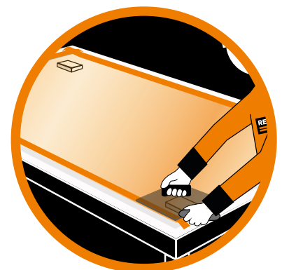
Figure 9. Mitre cut makes sure the tape from each side is in contact with the other.
