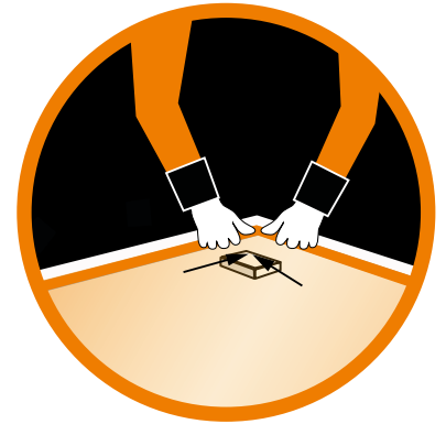
Figure 10. Corner finishing with pressure towards the splice from both sides.
